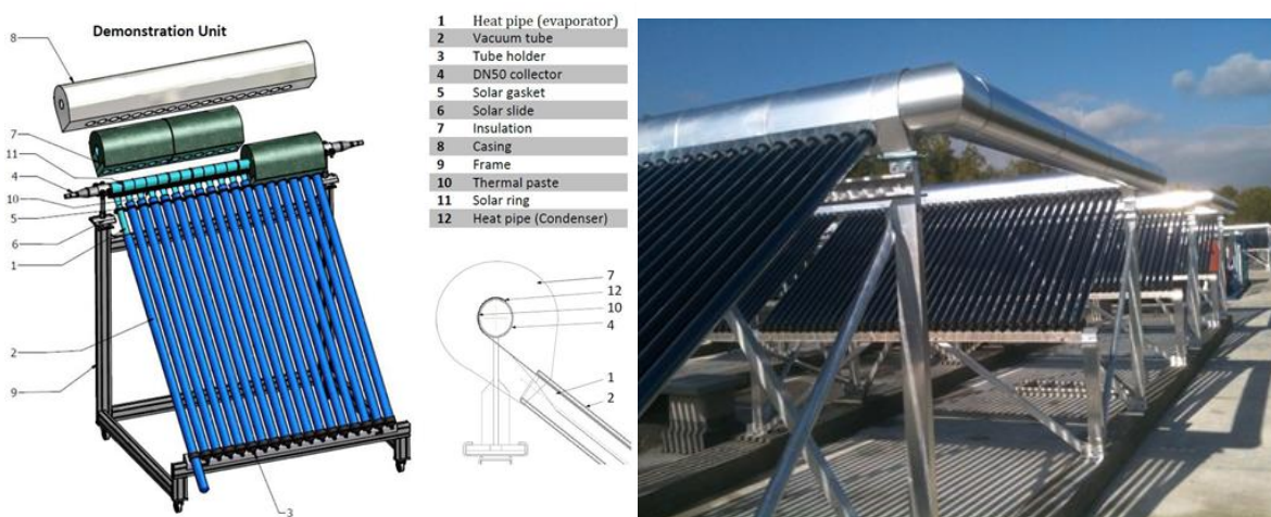
Figure 6: Solar thermal collectors – installation setup
