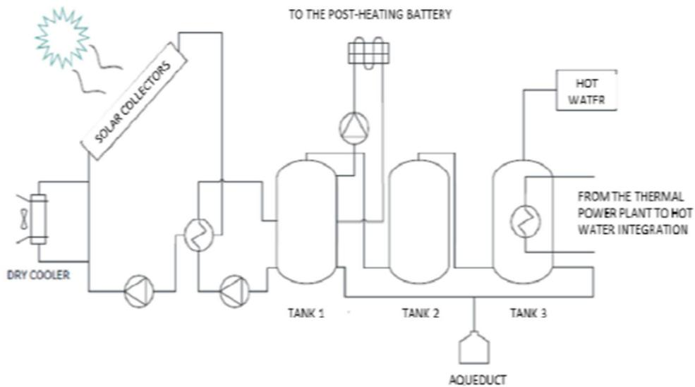
The existing solar power plant on the roof top of the Q2 building (scheme)
